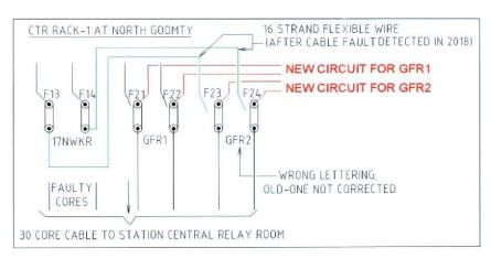
7.2.4.5 The S&T staff realized that they had disconnected the feed coming from the Crossover 17A/B to 17NWKR circuit, and instead connected 3GF RR circuit feed, which is normally available continuously, to 17NWKR circuit; thereby indication feed of Crossover 17A/B was disassociated from the status of the points at site. The following circuit diagram may please be referred in this regard:-
