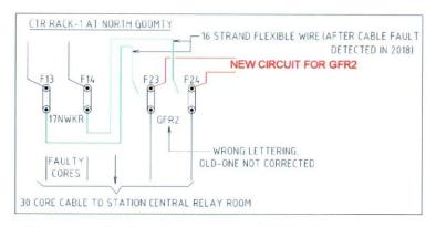
7.2.4.6 After the accident, at 23:28:51:046 hrs, 17NWK1R dropped automatically, picked up and finally dropped at 23:28:58:750 hrs. As per their deposition during the inquiry on 19.6.23, after noticing the mistake in the wiring mentioned above, second GFR (3GF RR) circuit, terminated on F23 & F24, was removed, and the originally released wires for 17NWKR were connected back. The following circuit diagram may please be referred in this regard:-
